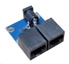
Power is distributed to nodes via the LCC network, along with the CAN bus. The recommendation is for a nominal 12 V power supply, which nodes will regulate to a lower voltage (typically 5 or 3.3 V) for their internal circuitry. A 12 V supply gives ample headroom for voltage drops along the network cables. Add up the current draw of the nodes connected to the network and use multiple PIPs if your LCC layout nodes require more than 1 A.
