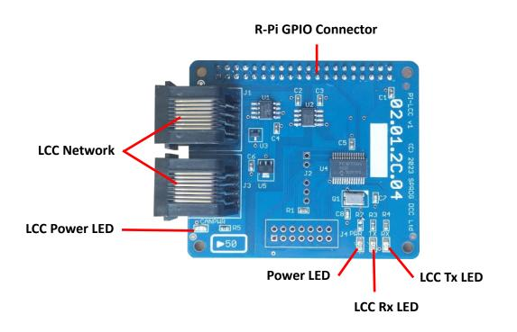
The LCC Power LED indicates the presence of power from the LCC network.
