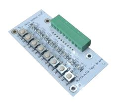
Connect a BUTTONLED module to the I/O of our LCC nodes during network setup and testing. Use the buttons to stimulate inputs to the node for event production. Use the LEDs to monitor outputs from the node from consumed events.
