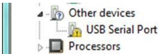
Right click on the USB Serial Prot entry, to repeat the driver update process, updating the drivers on this new entry, and following exactly the same steps.
